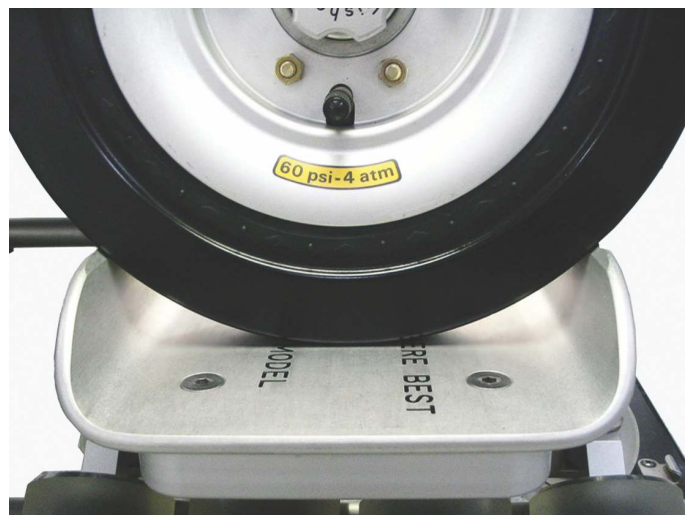
10 Dolly The channel properly fits the wheel. Notice the three points of contact.
