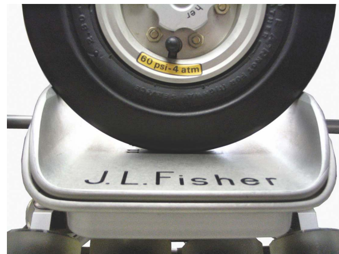
11 Dolly Note: The trays are used for the Model 11 dolly; allowing a perfect fit to the wheel. Notice the three points of contact.
