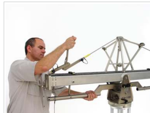
Tensioning the cables
