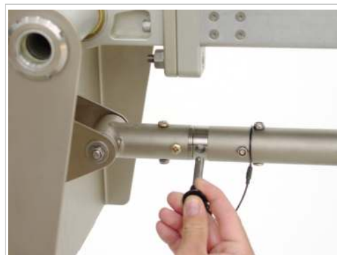
Locking pins secure all lower links
