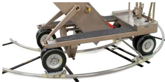
Model 9 Dolly shown with Skateboard Wheels (SBWS) on Round Curved Track (CR10)
