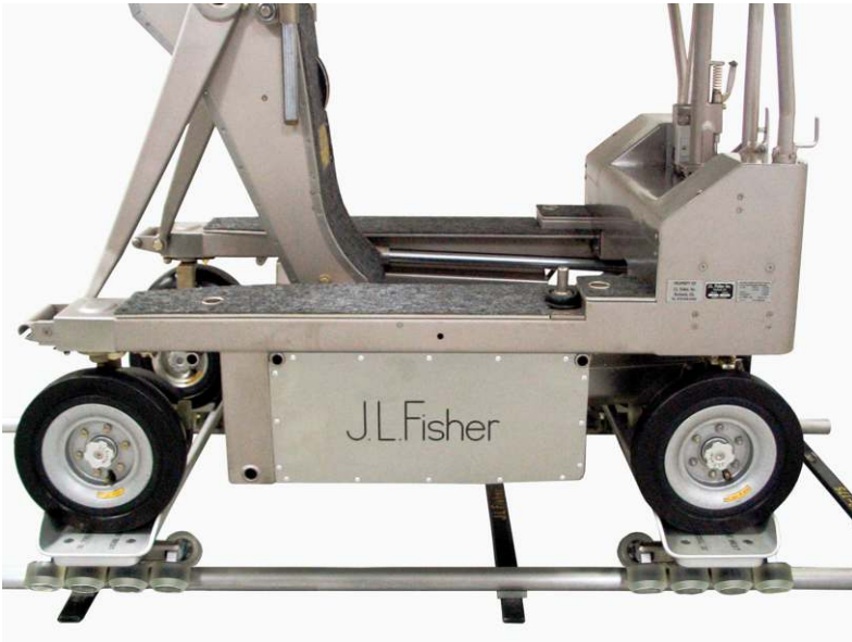
10 Dolly - mounted on standard 24.5 inch track (With no insert trays)
