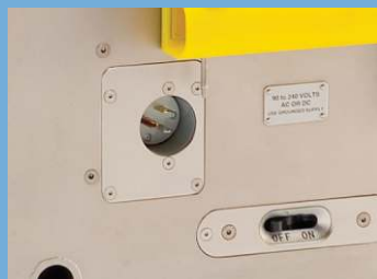
Power Requirements: 90 TO 240 VOLTS AC OR DC
